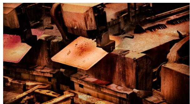
Anode casting in Harjavalta foundry (Credit: Boliden)
