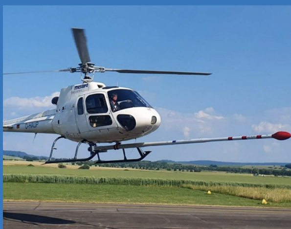
First ESA certified nose stinger for airborne surveys (Credit: terratec)
