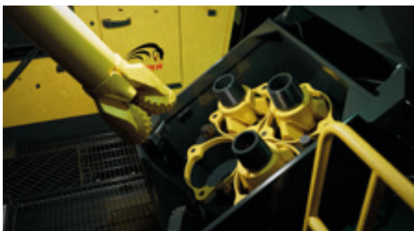
Automatic Bit Changer ABC (Credit: EPIROC)
