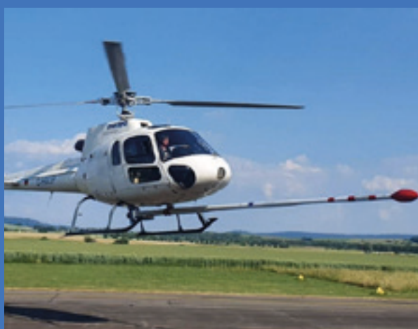
First ESA certified nose beam for airborne surveys (Credit: terratec)
